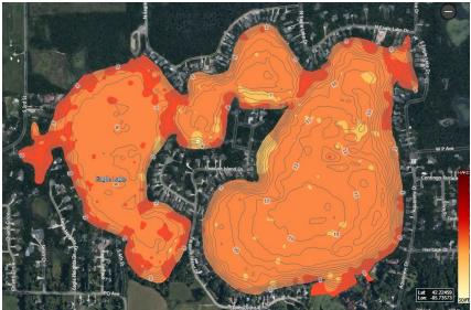
The overall hardness of the Lake bottom is improving despite the aeration pumps being disabled, as shown on the left
